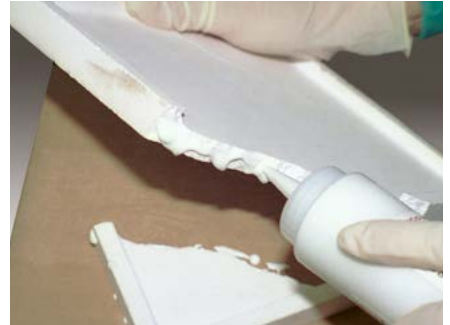
Cerabond™ 503 repairs furnace saggar plate.
