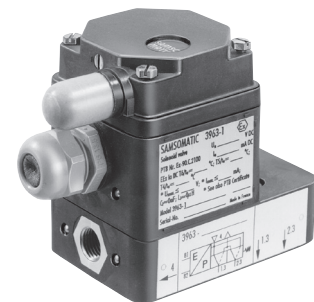
Fig. 1: 5/2-way solenoid valve · Actuated on one side · With spring return mechanism · K_{VS} 0.16 · G \frac{1}{4} connection
