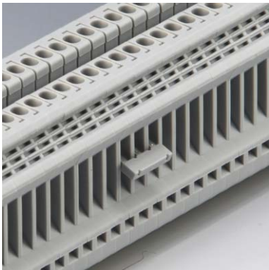
[Insertion bridge] It is installed on the above part of clamping conductors, which spares the cross channel of terminal blocks. The conductor's max. cross-section area needs to be decreased, when it is used.
