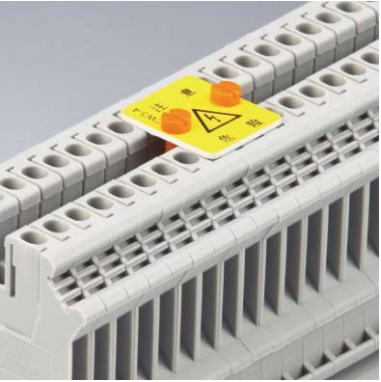
[Caution marking] It is fastened on conductor holder by plastic screw. It is used to identify and mark conductor holder which connects conductor wires. And protection cover plate with danger warning sign are also provided.
