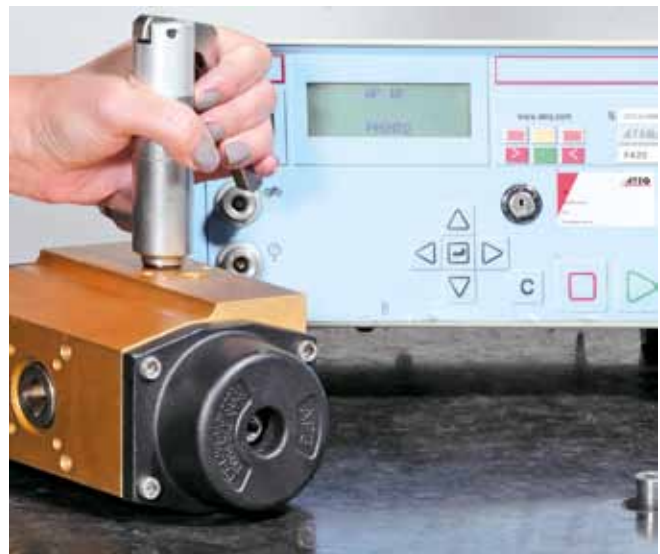
Leack test machine. For pneumatic rotary actuators.
