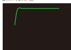
Second order step response (damping coefficient 0.7)
