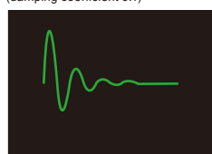
Second order impulse response (damping coefficient 0.2)
