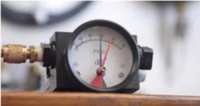
Follower Pointer: Shows Max Reading
