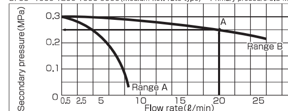
DFS3-1000-1200-1500-5000 (medium flow rate type) Primary pressure: 0.3 MPa
